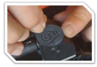
Hold the GutRad Key against the module's markings (circles) while turning on the system.
